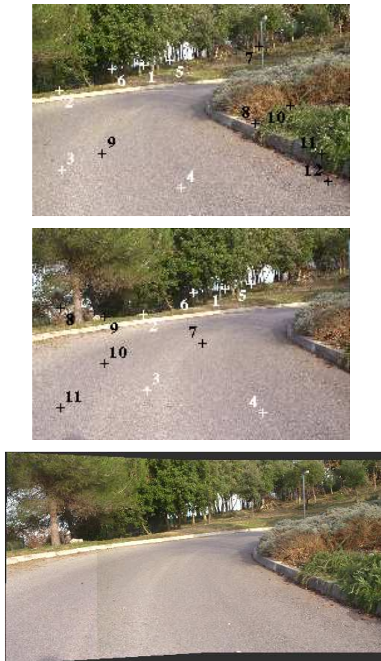
Figure 1: Image 1 at the top, image 2 in the middle, in black the extracted points, in white the points matched, the mosaic built with H_{opt} at the bottom.
